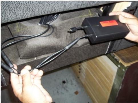
5- Insert the battery in the pocket and close the outside back. Recharge the battery with the electrical device (C).
