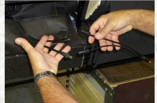
4-Connect the battery (A) within the plug of the dual output (B).
